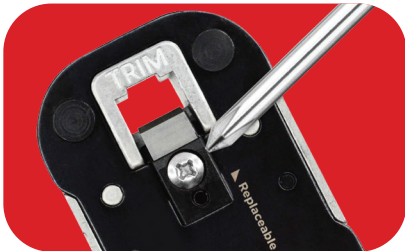
Quick Change Blade Cartridge Pre-Calibrated for Optimum Performance
